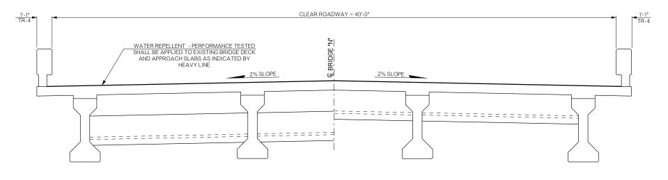
HALF SECTION AT INTERMEDIATE DIAPHRAGM
